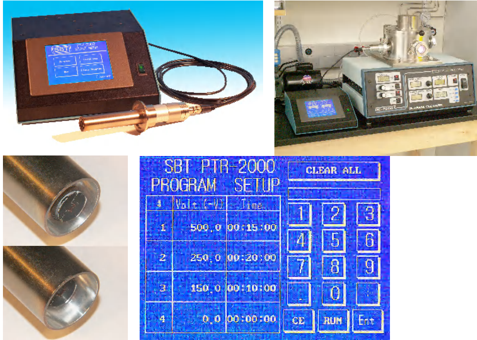
Figure 10 Model PTR-2000 Plasma Trimming™ Rod system. The PTR-2000 uses the same modified Fortress™ holder as the model PCPT. The programmable power supply can be programmed with up to four steps from 0 to -500V for 1 s to 24 hr.
